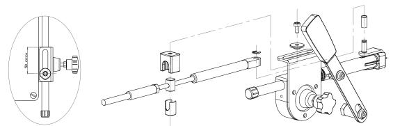
► Important: before the assembly, the throttle must be in minimum position and the gearbox must be in neutral position.
