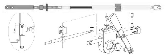
► Important: before the assembly, the throttle must be in minimum position and the gearbox must be in neutral position.
