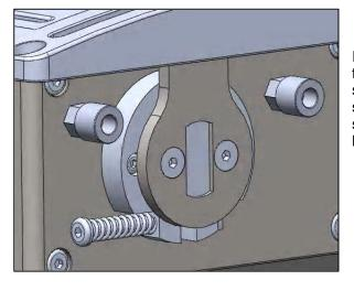
In order to adjust the friction of the lever, it is enough to tune the screw that you can find just behind the control lever, as shown in the picture on the left. With the help of an hexagon screw driver size 2,5 mm you can loosen or tighten the screw and the friction will become correspondingly softer or harder.
