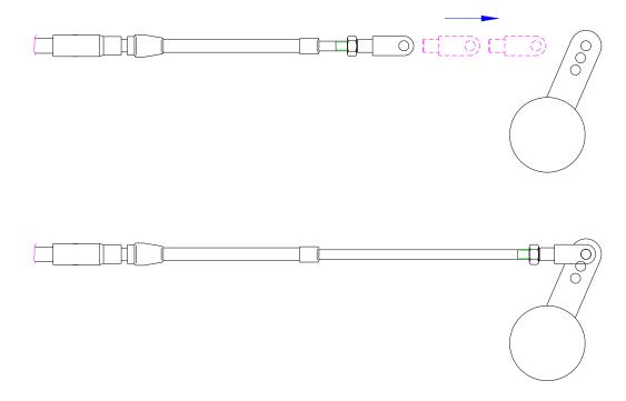
e. When the hole on the fork (or the ball joint) is aligned with the hole on the throttle lever (potentiometer), store the position with key "3".
