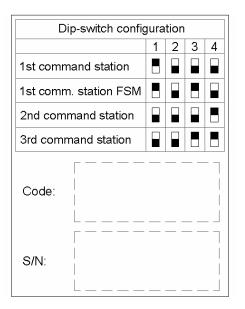
Under the base of the command station it is present the following label.
