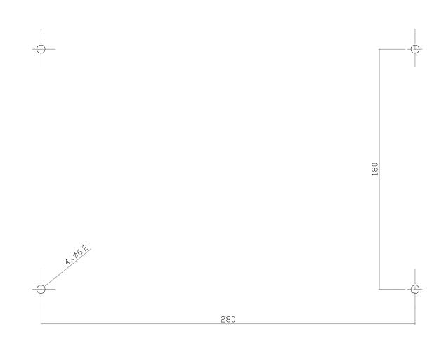
▶ Important: drilling mask is represented in scale 1:2
