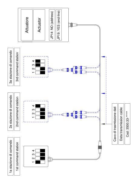
This installation scheme is valid for systems with up to 3 command stations and 1 engine with mechanical throttle, mechanical gearbox
